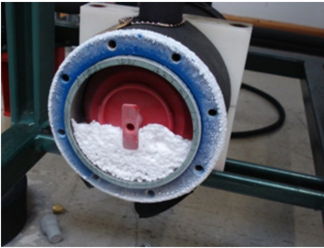
Figure 29. Example of dry ice formation in a drier
