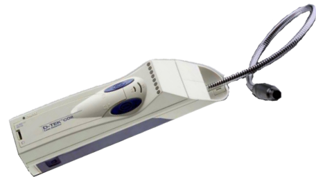
Figure 26. Example of an electronic leak detector suitable for R-744
